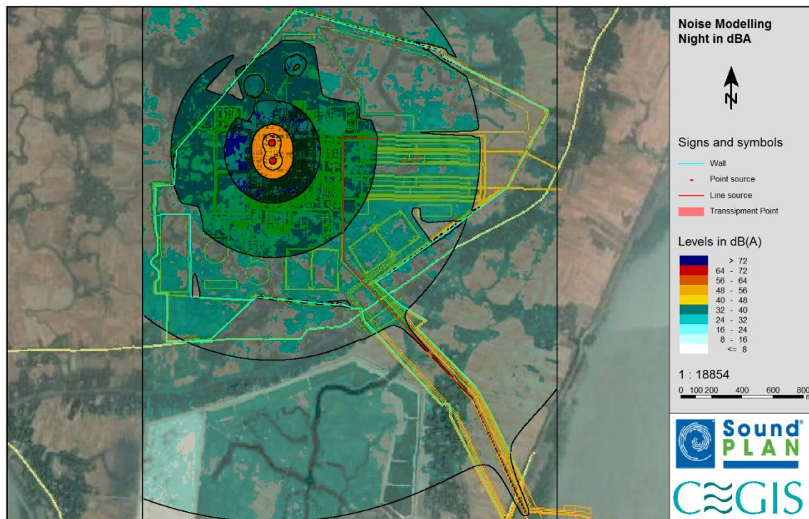
Figure 7.13: Propagation of noise from the sources (Night Time)
